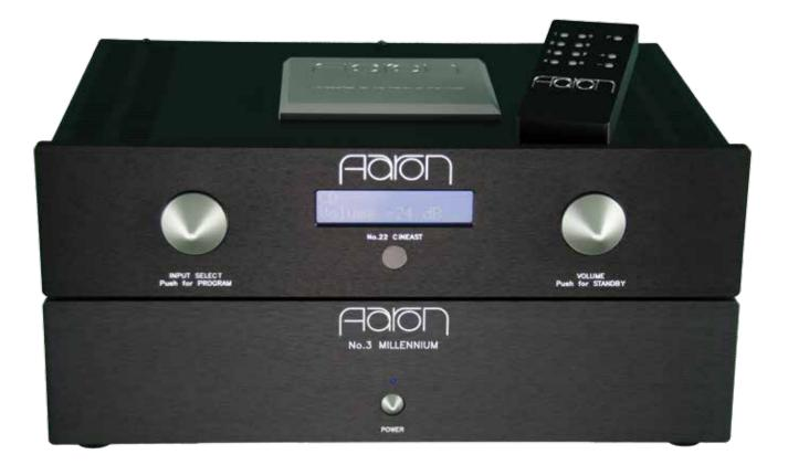
his is Aaron's pre-power system, but it's a system with a twist. While the No 3. Millennium power amplifier is a stereo design, the preamp – the No 22. Cineast – is designed to handle multichannel inputs alongside stereo line sources. While that would normally have audiophiles reaching for the 'off' button, the twist is there is no digital processing going on inside the preamp. It simply handles six channel sources, in the same
